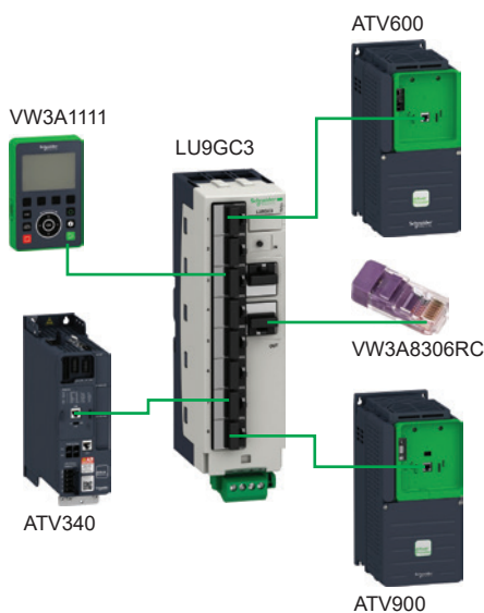
Example of multipoint screen architecture
